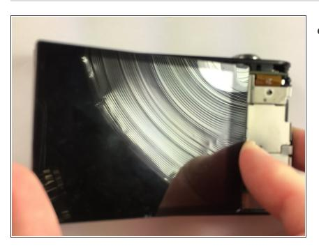
Remove the back LCD screen from its place carefully.
