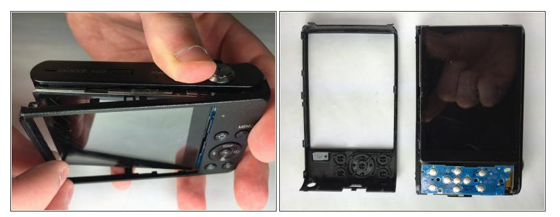
• Remove the back case of the camera carefully.
