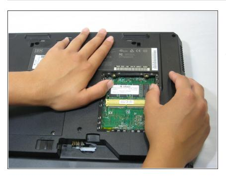
Remove RAM module by pressing the two metal pieces outward with your thumbs.
