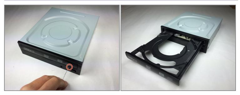
• Insert a paper clip into a small hole on the right side of the faceplate bellow the disc tray.
