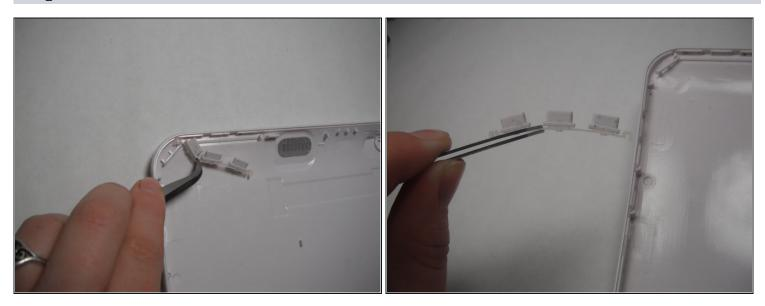
• With tweezers, pull the rubber holder from the back cover completely.
