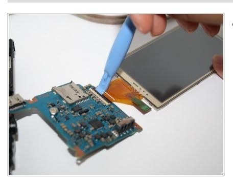
Next unclamp the connector to release the film strip and then you can replace your LCD screen.
