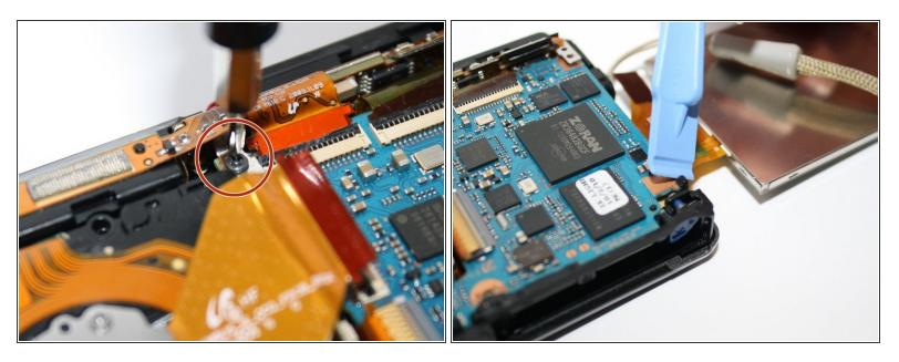
Remove the screw located above the center film strip. This holds the top frame in place.
