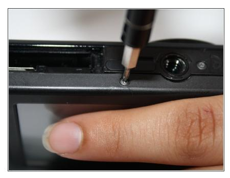
Begin with unscrewing the seven outer screws on the camera. There is one on each corner and then three at the bottom.
