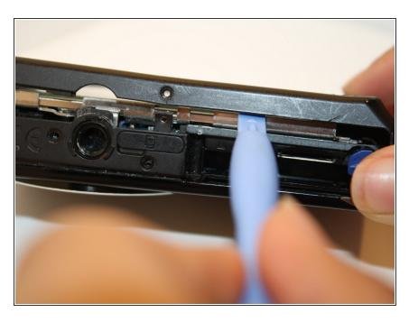
Now carefully pry open the back casing with the ifixit plastic opening tool.
