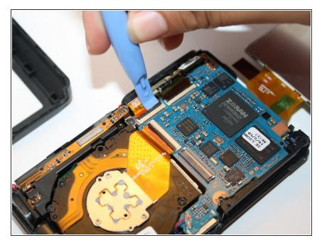
Unclip the four connectors to release the film strips.
