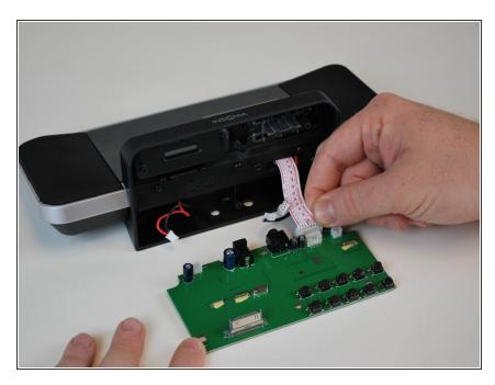
Remove the LCD screen plug last.
