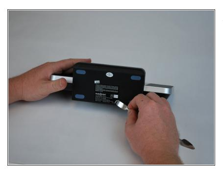
Begin by using a metal spudger to peel back the adhesive sticker and locate the 11mm screw beneath the sticker.
