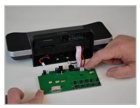
Remove the plug in the front of the lcd screen plug.
