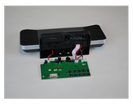
Locate the four plugs connecting the motherboard to the rest of the device.
