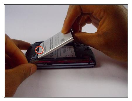
Once the old battery id removed, slide the new battery, with the positive/negative indicator facing up, in so that the contacts of the battery make contact with the contacts of the phone.
