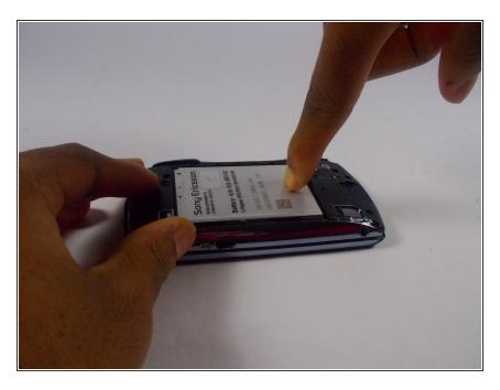
Lightly press the battery into the phone so that it is secure.
