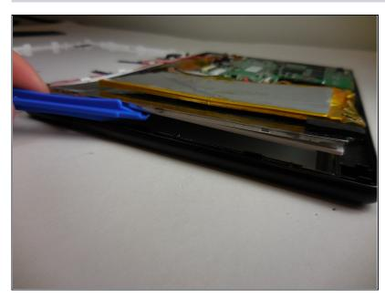
Use the plastic opening tool to pull the metal and plastic plates away from the interior of the tablet. Slowly pop each tab off until the plates are mostly separated from the base.
