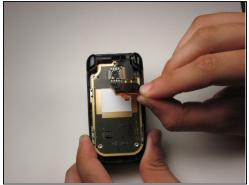
• Using a plastic opening tool, slowly pry the LCD display from the bottom, releasing it from the glue that is holding it to the board.
