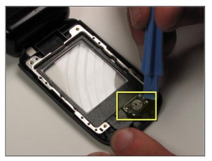
Using a case opening tool, gently pry the speaker in the bottom corner from the glue from right to left until it pops out.
