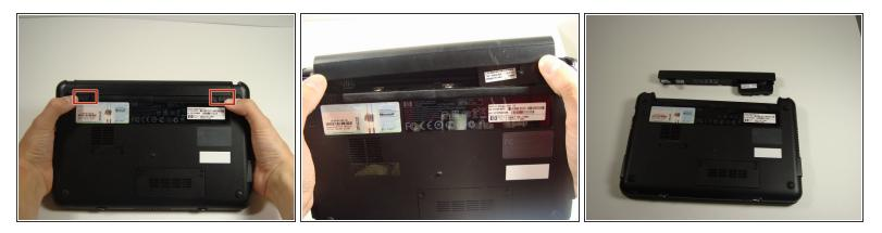
• Push both tabs inward simultaneously and slide the battery out.
