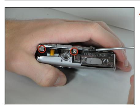
Remove 2 2.4mm screws on bottom.
