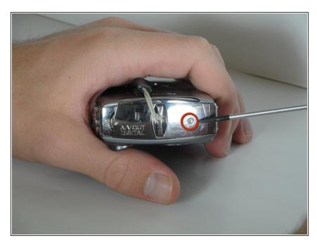
Remove one 4.7mm screw on the side with the AV output.
