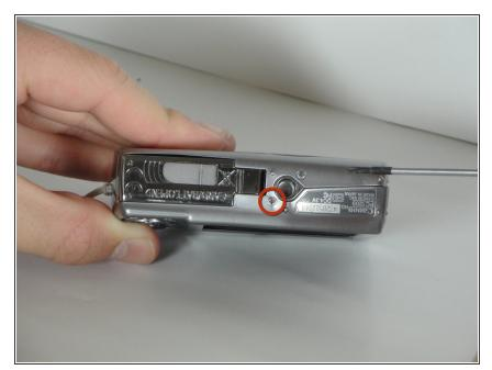
Remove one 2.25mm screw on the bottom.
