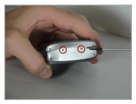
Remove two 2.25mm screws on the right side looking from the front.
