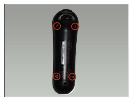
There are four screws located on the bottom of the controller. Located right above the bottom left screw is a reset switch, in case you need to resync the device to your PlayStation console.
