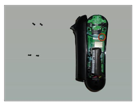
There is one ribbon cable connecting the two trigger buttons to the main board. It is easily removed with a little tug.
