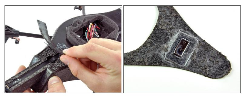
• The arduous task of peeling the protection blister from the body reveals the camera ribbon cable and the second magnet that holds the hull in place.
