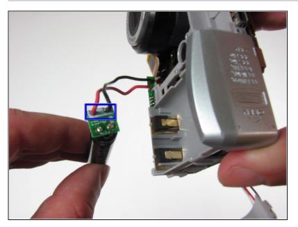
De-solder the connections at the base of the capacitor
