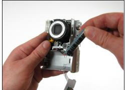
• Grasp the capacitor, carefully remove it from its holder, and place it off to the side.
