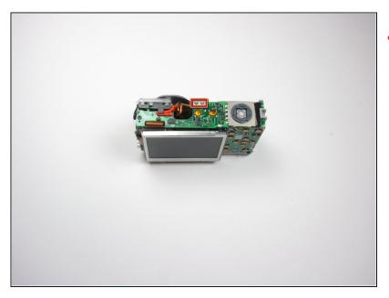
⚠ Do not touch the capacitor contact points for any reason. This will result in a severe shock.
