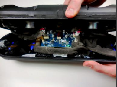
Pull apart the front casing from the back casing, slowly. Try to avoid any tension on any of the connected cables.
