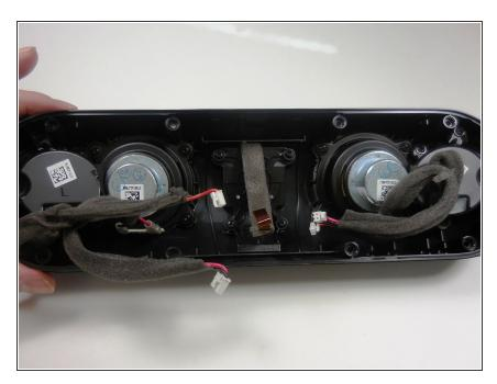
Separate the front case with the speakers and 'b' button from the mother board housing.
