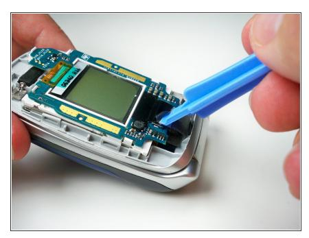
Use a plastic opening tool to lift the black tape off of the ribbon cable connector.
