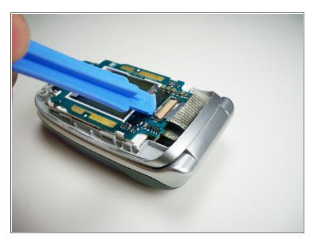
Lift the ribbon cable connector lock using a plastic opening tool.
