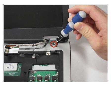
Remove the 8.6 mm screw on left side of upper case.
