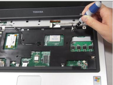
Remove the 3.76mm screw from the ground wire.
