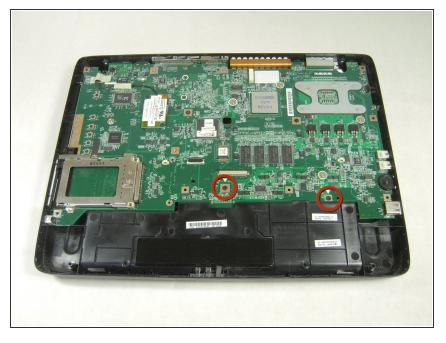
Using the Phillips Screwdriver, remove the two 8.6 mm screws from the front edge of the motherboard.
