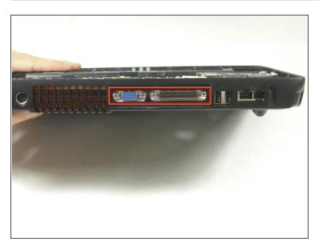
Remove the four screws holding the ports to the rear panel using the 3/16" Wrench.
