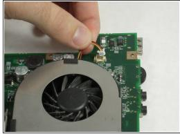
Remove cables connecting the fans with the motherboard.
