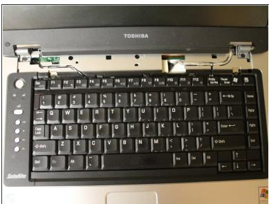
Remove the top panel by popping the panel out the top left socket, then do the same with the right side.
