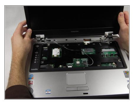
Lift up the display assembly to remove it.
