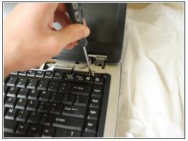
Remove the two 3.67 mm screws from the top corners of the keyboard.
