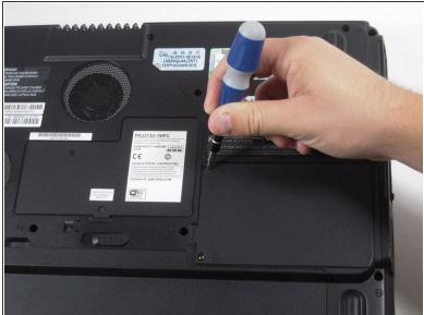
Remove the two 5.62 mm screws from the optical drive cover.
