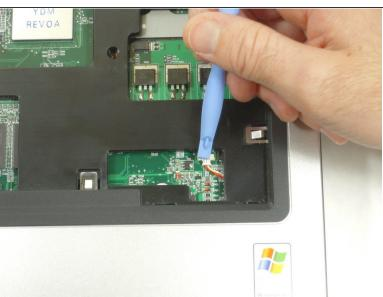
Use the plastic opening tool to remove the two speaker wire connectors and the trackpad connector from the motherboard.
