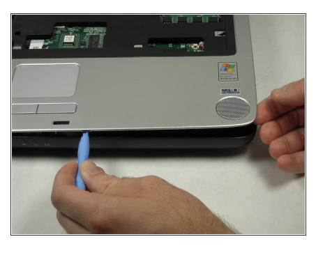
With the plastic opening tool, pry around the entire laptop to separate the upper case.
