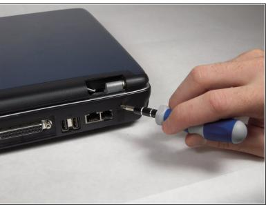
Remove two 8.6 mm screws on the back corners of the laptop.
