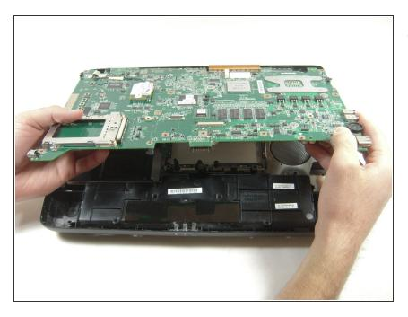
Lift the motherboard's front edge up and then slide it forward.
