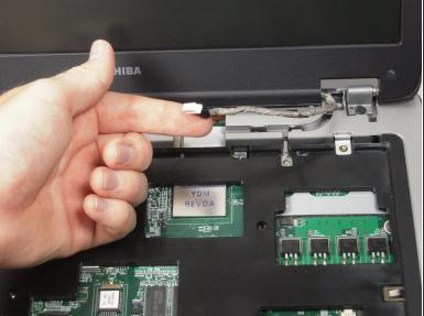
Use the plastic opening tool to remove the wire.
