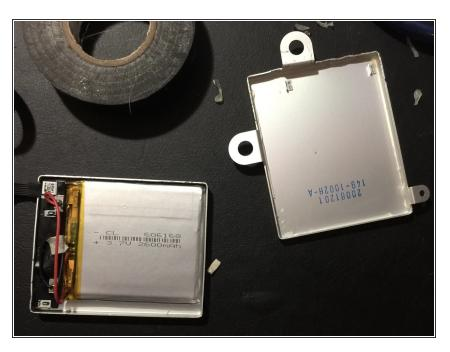
If you have been unable to recondition the cell to a state where the RAID card will accept it, the cell will need to be replaced. (It is also possible the RAID card is faulty, but it's much more likely to be the battery)
