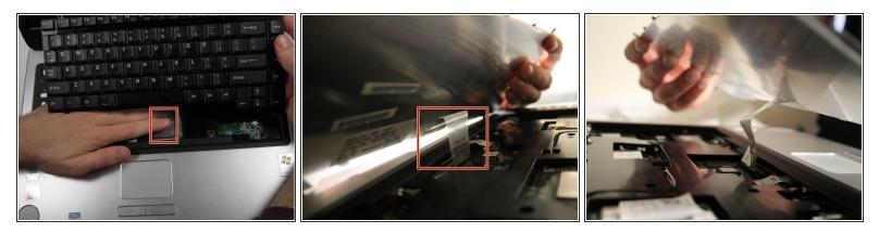
• Remove the cable connecting the keyboard with the motherboard.
