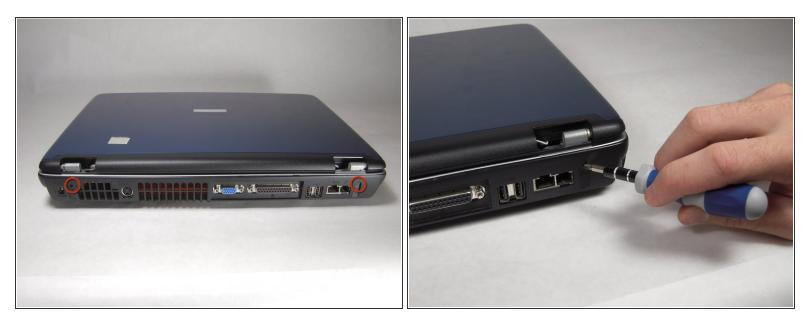
• Remove two 8.6 mm screws on the back corners of the laptop.
