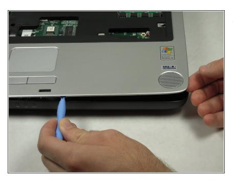
• With the plastic opening tool, pry around the entire laptop to separate the upper case.
