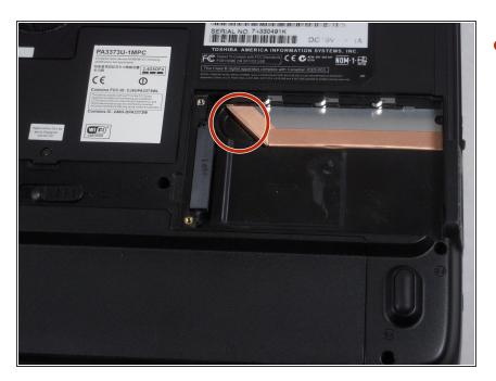
Using the inset divot, push the optical drive out of the laptop to remove.
