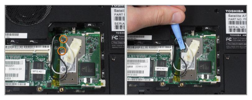
Use a plastic opening tool to disconnect the black and white antenna cable's connectors from the Wi-Fi card.
