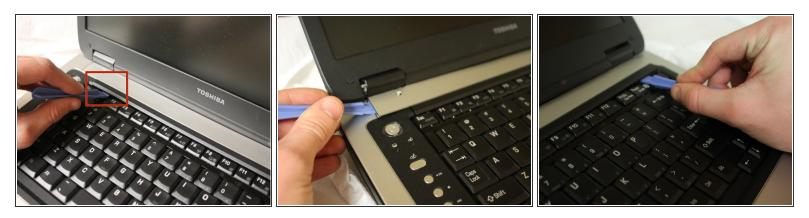
• Use the plastic opening tool to lift up the top panel all the way along the keyboard until it loosens.
