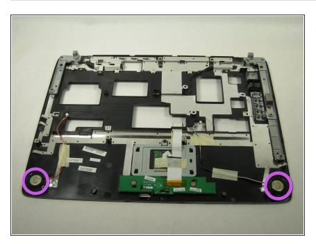
• Locate the two speakers on the underside of the upper case.
