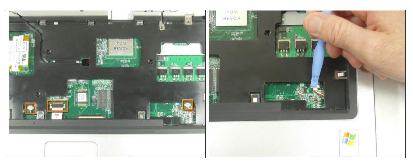
Use the plastic opening tool to remove the two speaker wire connectors and the trackpad connector from the motherboard.
