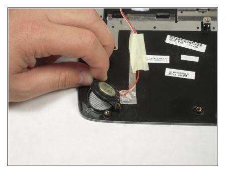
• Lift the speakers from the case to remove.
