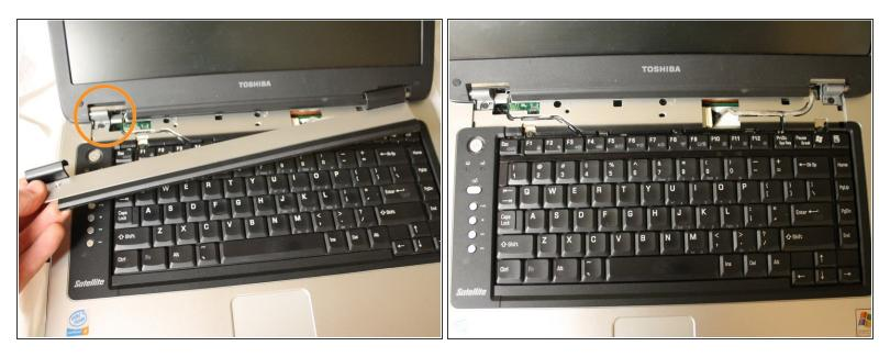
Remove the top panel by popping the panel out the top left socket, then do the same with the right side.
