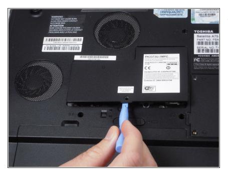
• Lift up the cover panel using a plastic opening tool.
