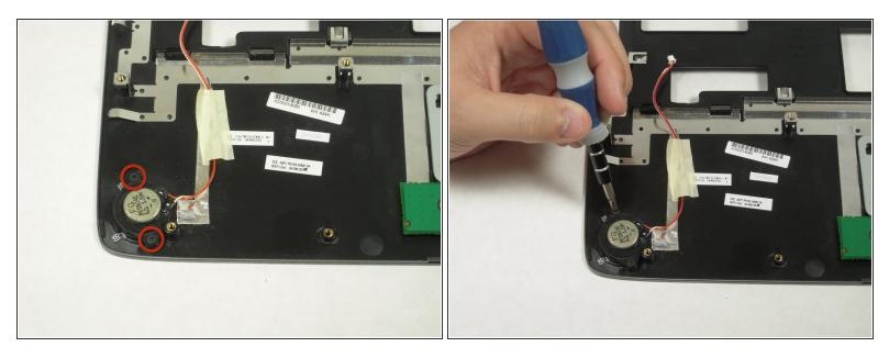
• Remove two screws from each speaker with the Phillips Screwdriver.
