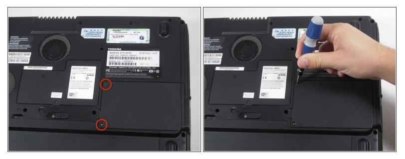
• Remove the two 5.62 mm screws from the optical drive cover.
