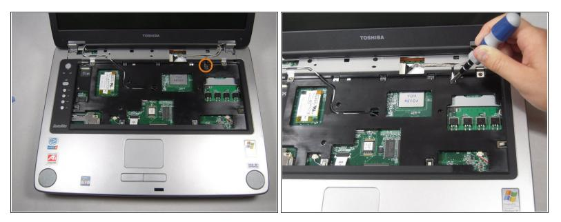
• Remove the 3.76mm screw from the ground wire.
