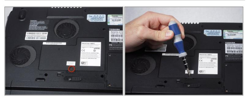
Remove the 5.75 mm screw from the cover panel.
