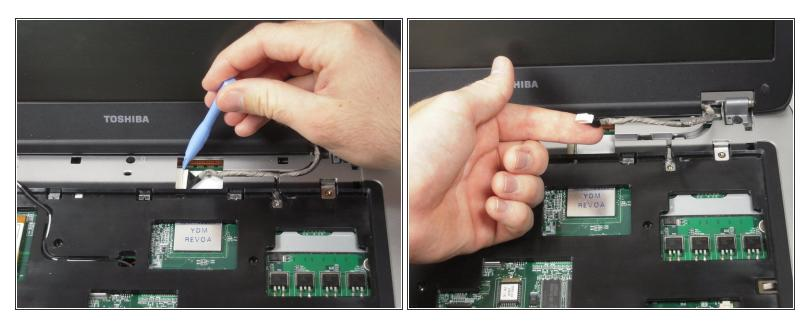
• Use the plastic opening tool to remove the wire.
