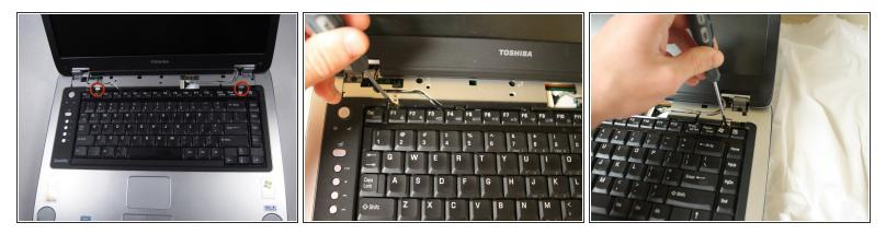
• Remove the two 3.67 mm screws from the top corners of the keyboard.
