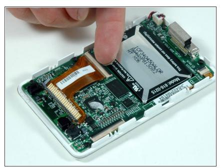
Use the tip of your finger or a spudger to carefully flip up the black connector securing the hard drive cable to the logic board. Note that the black retaining clip flips 90 degrees toward vertical, in the direction of the cable.
