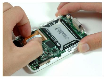
• Pull the orange hard drive cable directly out of its connector.
