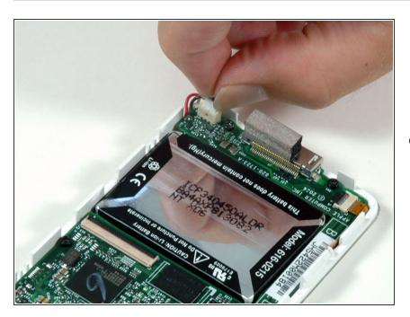
Carefully disconnect the white battery connector from the logic board. Be sure to pull only on the
