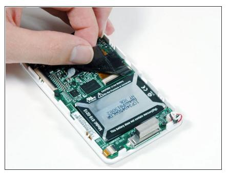
• Peel up the black adhesive strip covering the hard drive ribbon cable.
