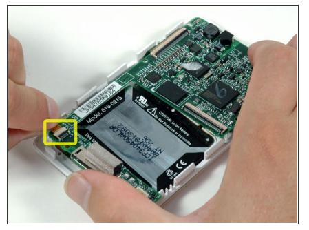
Slide the orange click wheel ribbon cable out of its connector. You must unlock this connector before sliding the ribbon cable out. The locking mechanism is on the opposite side of where the cable is inserted - it swivels upwards 90 degrees. Use a plastic spudger to lift the locking mechanism.
