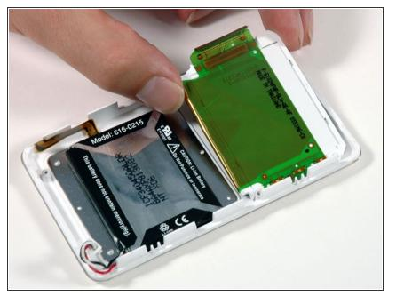
Lift the display panel out of the iPod. There may be some mild adhesive connecting the display to the front panel.
