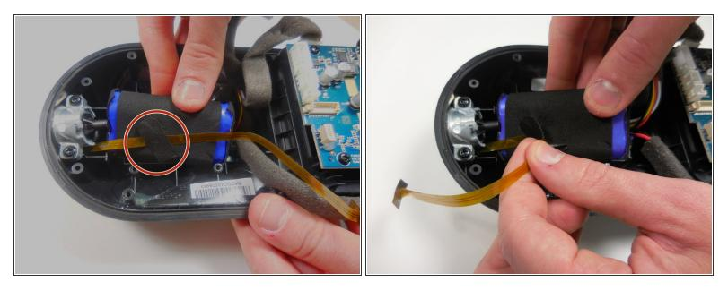
Remove the padded sticker holding down the ribbon cable to one of the batteries.
