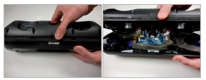
Pull apart the front casing from the back casing, slowly. Try to avoid any tension on any of the connected cables.
