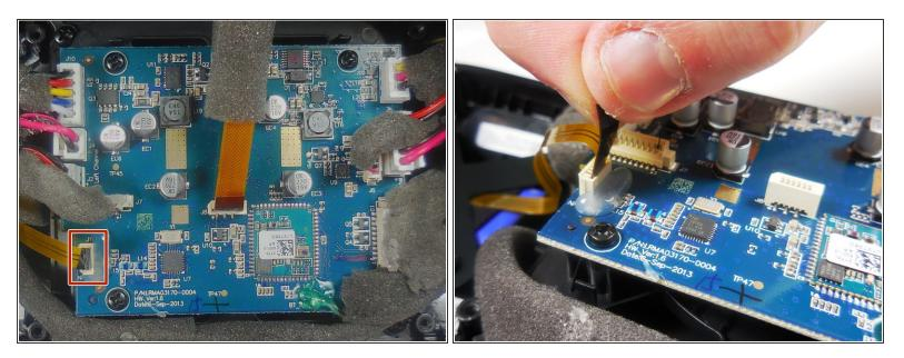
• Gently pull up on the plastic tab at the base of the ribbon cable to remove it from the motherboard.
