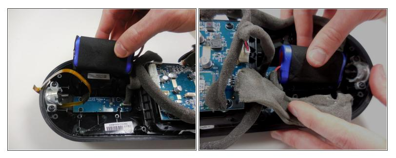
• Lift straight up from the casing to remove each batteries from their tight spaces.
