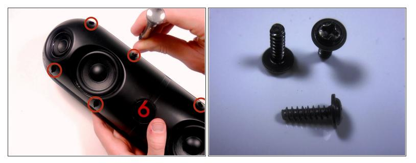
Using a Phillips #2 screwdriver, remove the 8 (10mm maxi-loc Phillips #2) screws that hold the casing together.
