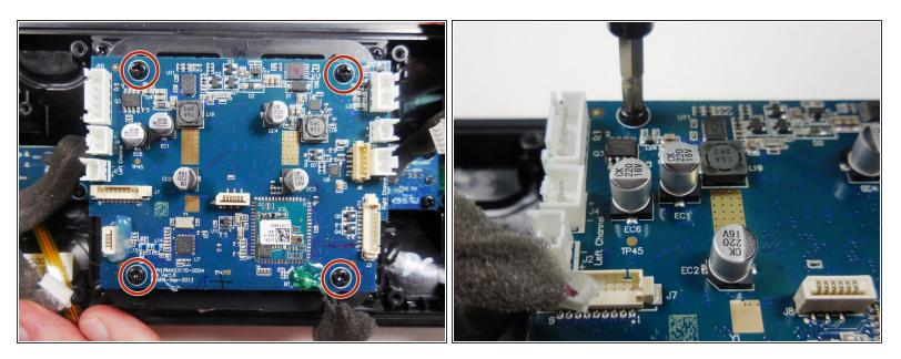
Using a Phillips #2 screwdriver, unscrew the 4 (8mm pan head Phillips #2) screws holding the motherboard onto the case. They are located in the four corners of the board.
