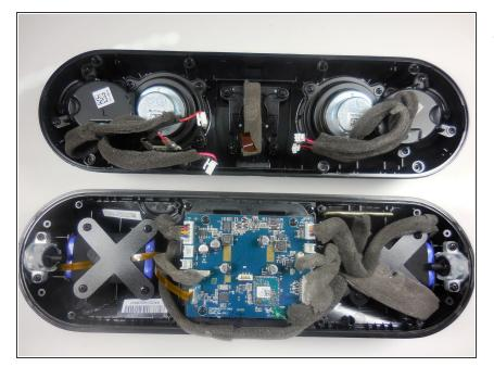
• Set the half of the device containing speakers to the side.
