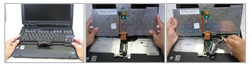
A Be careful not to pull out the keyboard carelessly; there is a connector underneath it!
