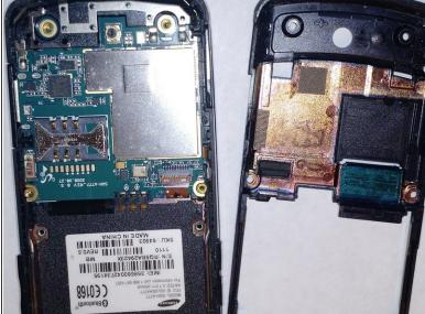
Using a spudger pry the back cover off carefully.
