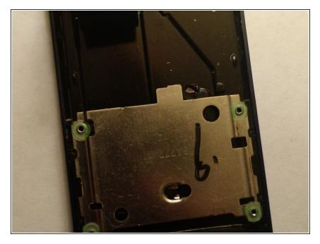
Pry starting at the bottom with a spudger. Remove the cover. This will require some force and a guitar pick.
