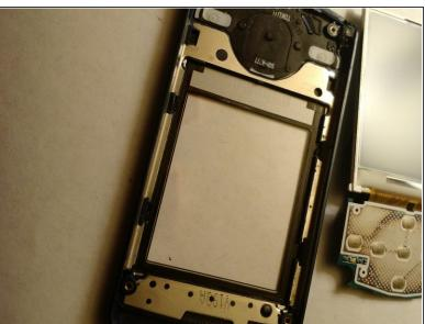
Using a guitar pick, carefully pry up the LCD shield plate from the sides.
