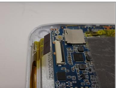
Gently remove the ZIF cable from the connector.
