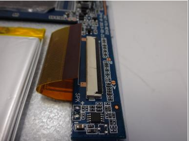
Disconnect the second ZIF connector using the same method detailed earlier.
