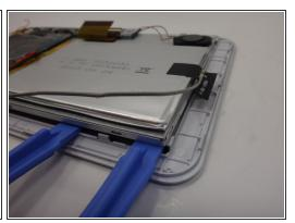
Use a third plastic opening tool to pry at the corner of the tablet and pop off the metal backing.
