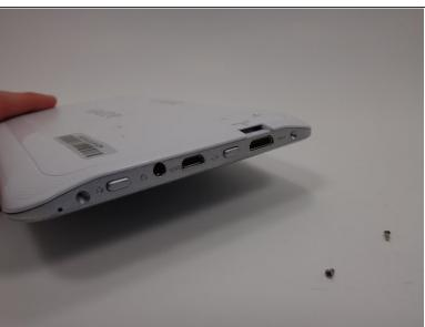
Use a Phillips #00 screwdriver to remove the two 4mm screws found on the top edge of the tablet near the power button.
