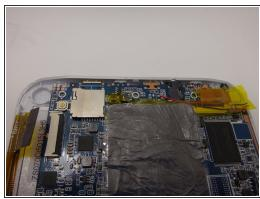
Remove the three 4mm Phillips #00 screws securing the motherboard in place.
