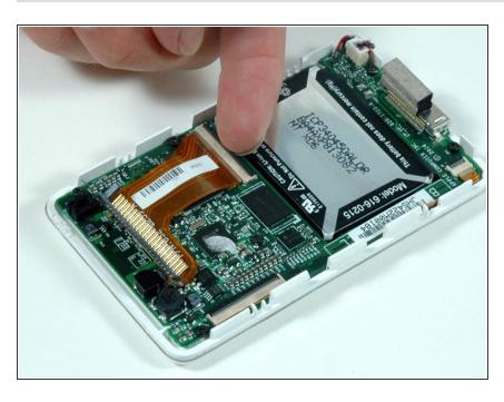
Use the tip of your finger or a spudger to carefully flip up the black connector securing the hard drive cable to the logic board. Note that the black retaining clip flips 90 degrees toward vertical, in the direction of the cable.
