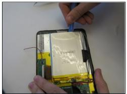
• Remove the battery pack by carefully prying the battery back from the front cover. Then remove the wires connecting the battery to the motherboard at the motherboard using the <u>tweezers</u>.
