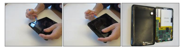
• Remove back cover with lever tool, exposing the battery and motherboard.
