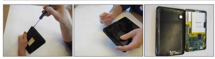
• Remove two 2.4mm x 4mm screws from bottom of the tablet with Phillips #00 Screwdriver.
