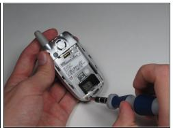
At the corners of the phone, remove all four 6.0 mm Torx screws.
