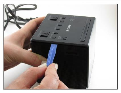
Use the opening tool to pry apart the edges of the top and side portions of the device.
