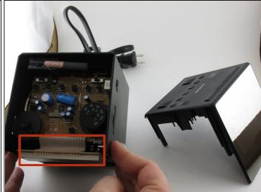
Separate the device by gently pulling up on the top portion.
