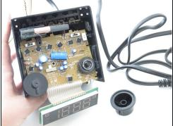
Remove the tuner dial by pulling it off of the motherboard. This can take a little force to remove.
