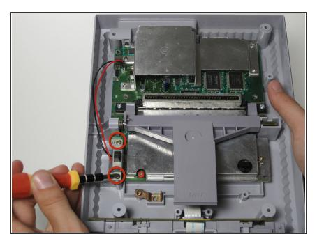
Remove the two 11.7 mm Phillips #2 screws connecting the power switch to the motherboard.
