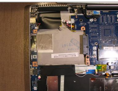
Remove the hard drive by slightly lifting it up on the left side and slightly pulling it to the left carefully untill it pops out.
