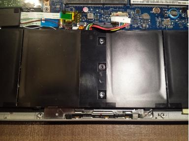
Remove the two battery screws.
