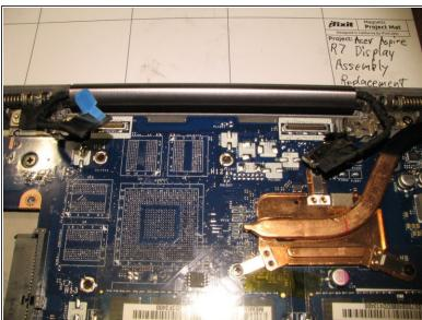
Disconnect the two display cables.
