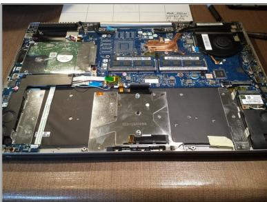
Remove the battery by lifting it up carfully.
