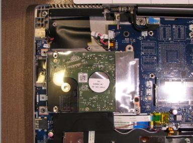
Remove the 2 top screws on the hard drive.
