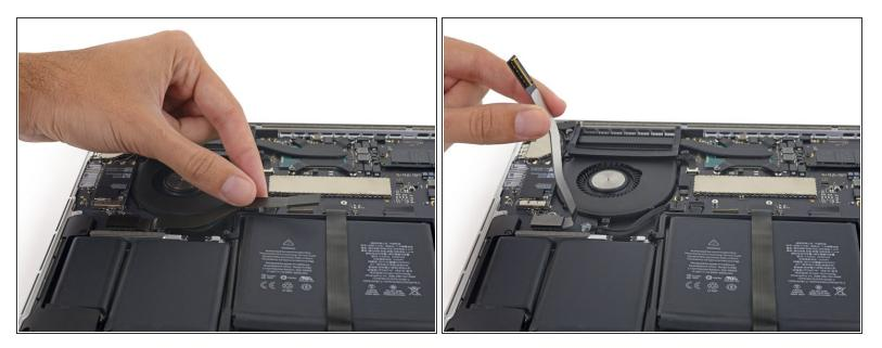
• Lift the logic board end of the I/O board cable straight up to bend it out of the way.
