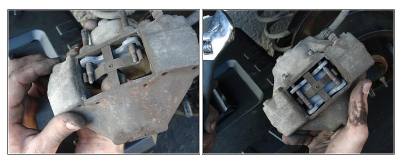
Verify that pins are inserted through caliper and brake pad holes and seated over the metal pin guides.
