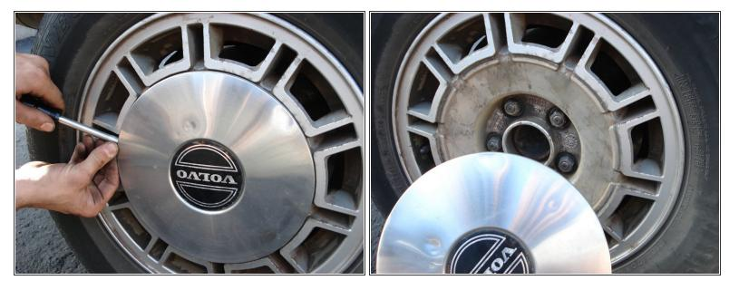
Pry off the front hub caps by placing a small flathead screwdriver between hubcap and rim and pulling the screwdriver and hubcap away from tire.
