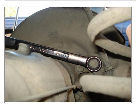
Remove upper and lower guide bolts on rear left and rear right brake calipers with 17mm crescent wrench.
