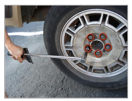
Loosen each of the five lug nuts on the rear left and rear right tires by turning them counter-clockwise with a 19mm socket wrench.
