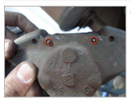
Locate the two rear brake pad retaining pins on each caliper.
