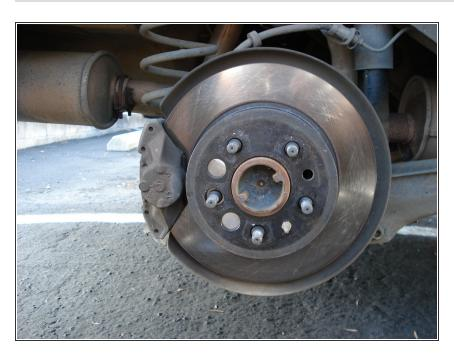
Remove tires by pulling directly away from car exposing rear brake disks and calipers.
