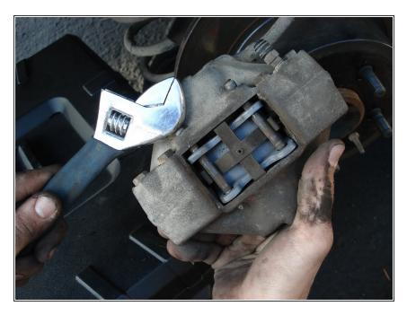
Tap pins through both rear brake pads and caliper using a wrench.
