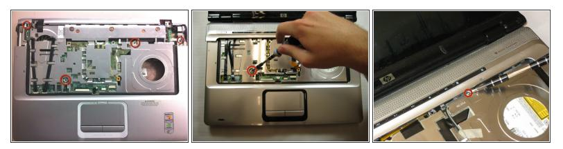
Remove the four 5.8 mm Phillips screws securing the top cover to the lower case.
