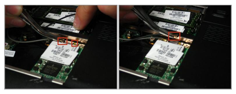
• Use a pair of tweezers to disconnect both antennas from their sockets on the wireless card. These are snap-on connectors, so simply pull them straight up to snap them off the studs on the card.
