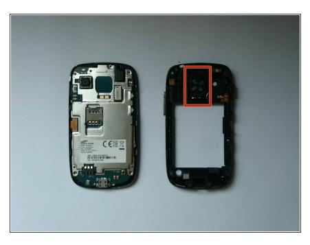
The Loudspeaker is located on the rear housing..
