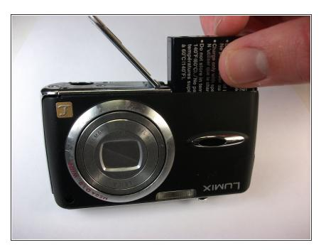
Remove the battery from the camera.
