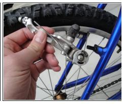
• Loosen the brake caliper bolt, and remove the brake caliper.
