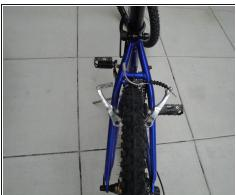
• Squeeze the calipers together, and remove the brake cable.
