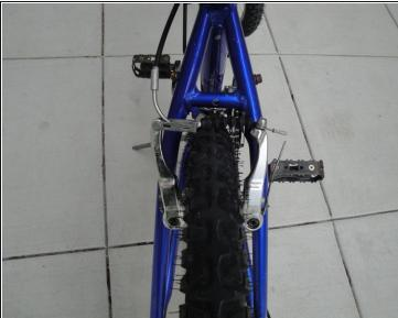
Reattach the brake cable to the calipers.
