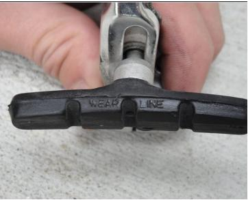
Inspect the brake pad. If the pad has worn down past the "wear line", then it needs to be replaced.
