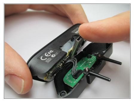
Pull back on the controller USB connector with your finger to separate the main adapter circuit board from the rubber mold in the button panel.
