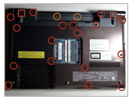
Remove all screws from the bottom cover. There are three types of screws. Marked here with Red Circles, Red Squares and Orange Circles.
