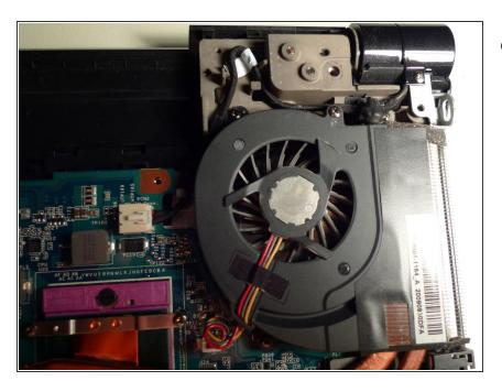
Fire up the air compressor and blow out dust from the fan and heatsinks.
