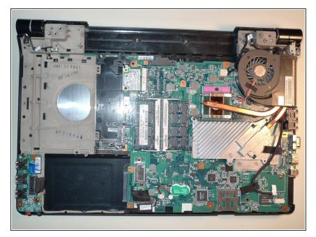
Carefully remove the cover, by unpopping it with a slim flathead, slide it out away from the RJ-45, HDMI and VGA ports.
