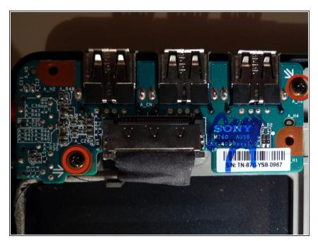
The audio/usb interface card is now within reach. Just remove the two screws and carefully slide out the flat connector to remove the card.
