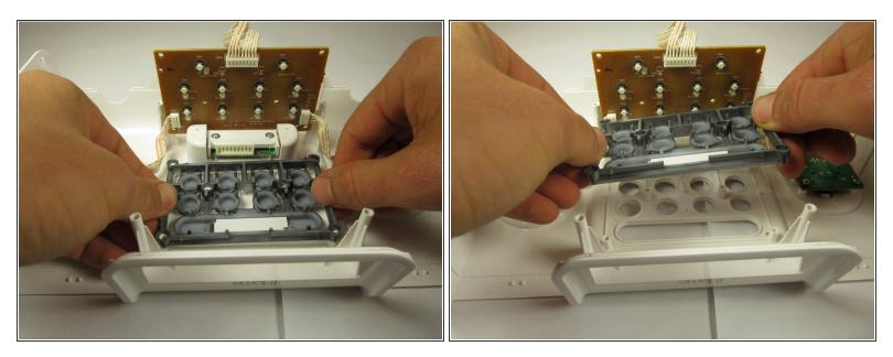
• Firmly grasp the sides of the button grouping and lift up.
