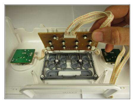
• Lift the circuit board up and away from the body.
