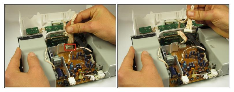
Unplug the narrow 9-pin connector from the motherboard.
