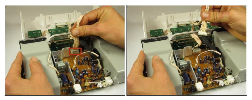
Unplug the narrow 9-pin connector from the motherboard.
