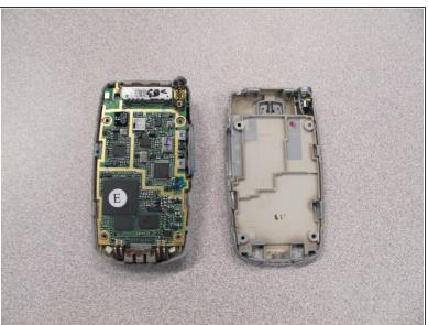
Pull the back cover straight off the phone using your thumb and forefinger.
