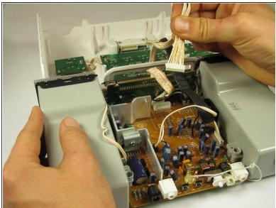
Unplug the narrow 9-pin connector from the motherboard.
