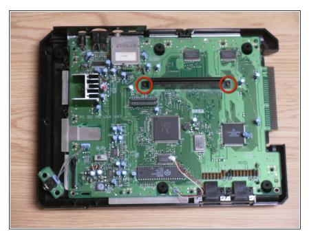
Remove two black screws on the left and right sides of the cartridge slot.
