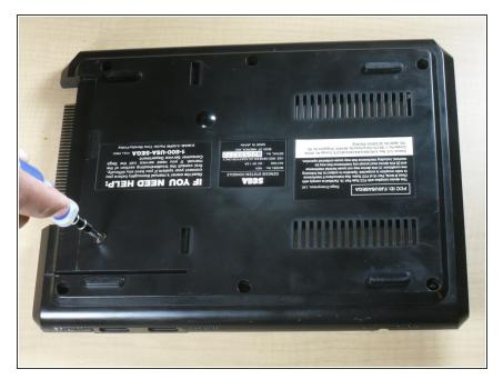
Remove single black screw from the outside of the bottom cover, using a Philips screwdriver.
