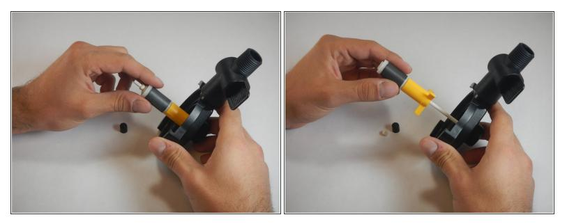
• Hold the impeller cover with one hand and the impeller with the other. Slide the impeller out.
