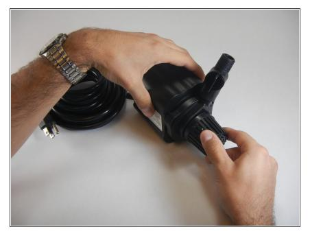
Hold the inlet screen and rotate it counterclockwise to unscrew it. It is helpful to remove the inlet screen so that it is not damaged during the replacement process.
