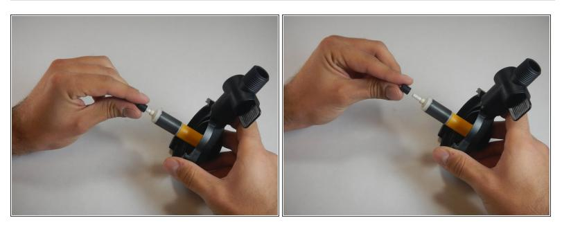
Remove the rubber stop that is attached to the tube that runs through the middle of the impeller.
