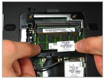
Under the first RAM stick is another. Remove it in the same way by pushing the silver tabs away and down from the RAM stick and remove the RAM once it pops up.
