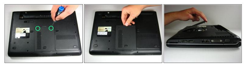
Remove the two screws from the memory shield and lift up. The screws will remain into the shield
