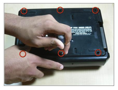
Remove the six screws from the underside of the console with a Phillips #1 screwdriver.
