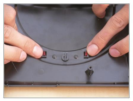
• Remove plastic "Power / On" cover by pushing tabs together.
