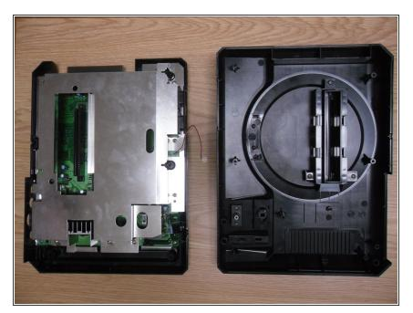
• Separate the main board from the outer case.
