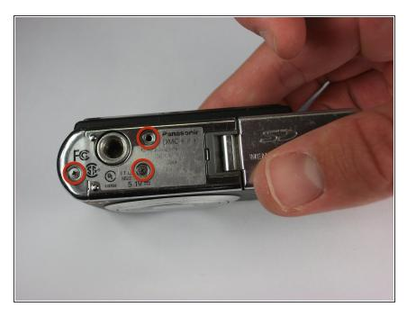
Remove the three 4.6 mm screws on the bottom of the camera using a Phillips #00 screwdriver.
