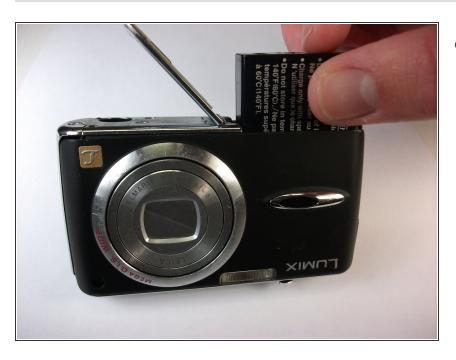
Remove the battery from the camera.
