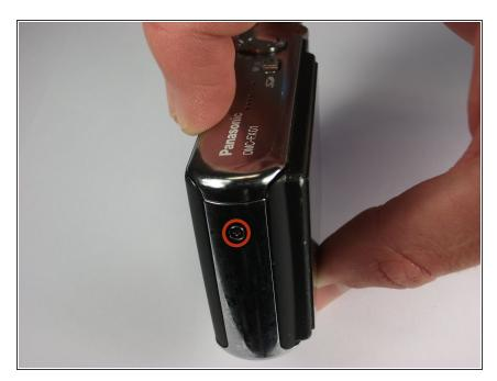
Remove the single 3.2 mm screw on the left side of the camera using a Phillips #00 screwdriver.
