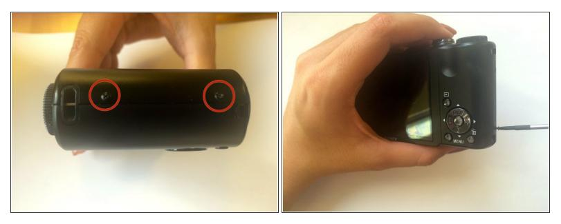
• Use the Phillips #00 screwdriver to remove the two screws located on the right side of the camera.
