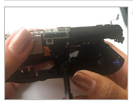
Pull off front outer shell by pushing off from left side.
