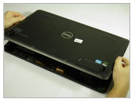
Gently lift the back cover off the device. The back cover should come off easily.
