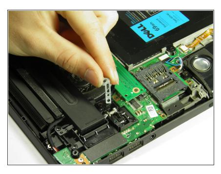
Remove the silver metal piece holding the support feet down.
