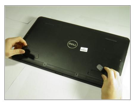
Gently flip out support feet located near the bottom of device.
