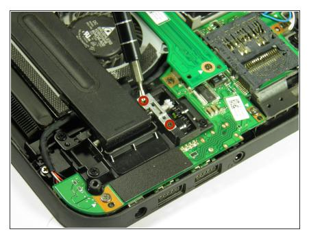
Remove the two silver 3mm screws with a Phillips 00 screwdriver.
